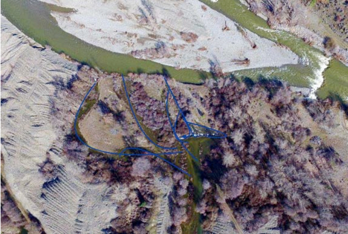
Drone Photo Joey Howard 2/11/2017. Blue lines represent the multiple flow pathways at high flows.
